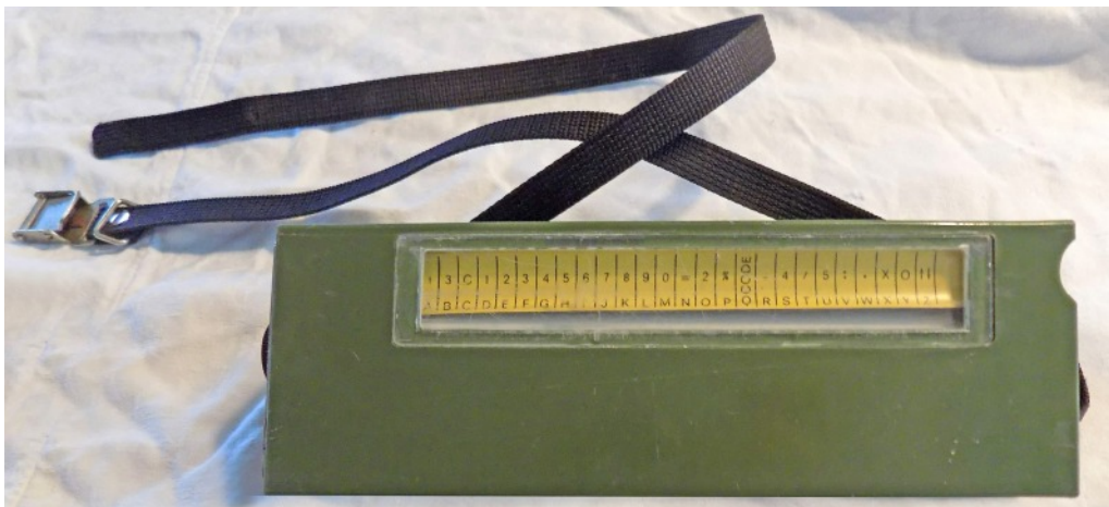
Issued with VR 17 stations was a remarkable manually operated cipher unit. It was comprised of a retractable tape measure printed with the alphabet, numbers and symbols, and a rotating drum. Not a high security and unbreakable cipher system, but for simple field use under any weather condition, without mechanical or electrical complexity, suitably only for immediate and short term use.
