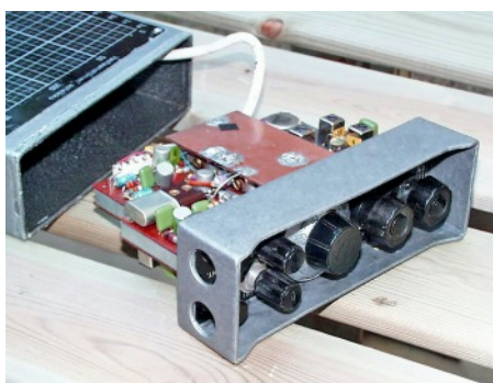
VR 17 transmitter receiver unit removed from its enclosure (left).
