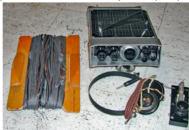
The main items of a VR 17 'Sipi' station (below).
