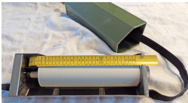
Internal view of the VR 17 cipher unit showing the printed tape measure and drum.
