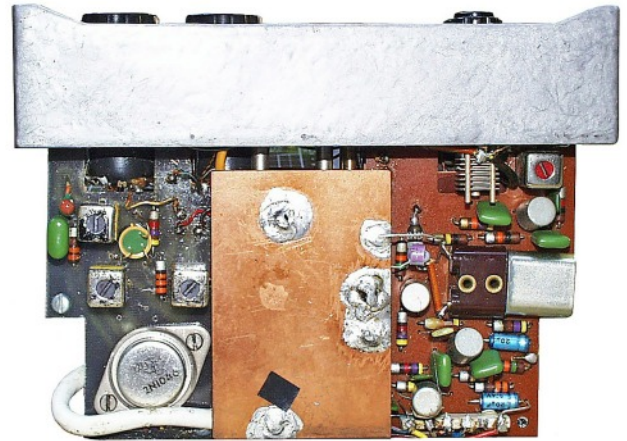
Internal view of the VR 17 opposite side with the transmitter board (left) and receiver board with BFO section, AF output, and 200kHz calibrator crystal (right).
